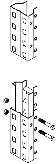
Slide the Splice Kit inside the lower frame so the top two holes of the frame line up with the lower two holes of the kit plate.
