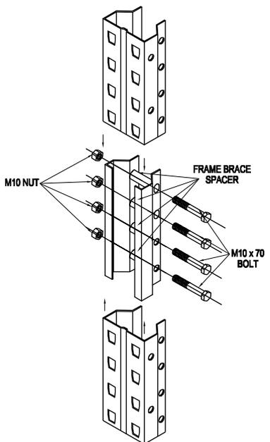
Splicers enable you to increase the height of your pallet racking by joining 2 frame sections together.
