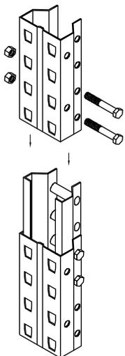
Slide the upper frame over the exposed kit and repeat Step One by inserting the frame spacer and bolts.
