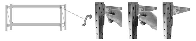
To ensure beams stay securely in place, you must install a beam locking pin into each end of every beam used (every shelf level requires 4 locking pins). Once the beam is located at the correct level and firmly inserted into the tapered post holes, the small hole in the beam indicated below will line up with a matching hole in the post. This will allow the 'S' shaped locking pin to be inserted (thin end first) until the head stops against the beam.
