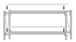
Place the particleboard, wire decks or galvanised shelves onto the top inner lip of each pair of beams as shown in the diagram
