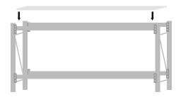
Starting at the upper level, place the particleboard onto the top inner lip of each pair of beams as shown in the diagram.
