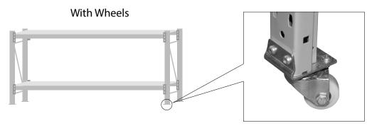
If required, fix frames to the floor through the hole in each foot with appropriate floor fixings (expansion bolts for concrete or screws for wood). Fixings are an optional accessory and not supplied as standard.
