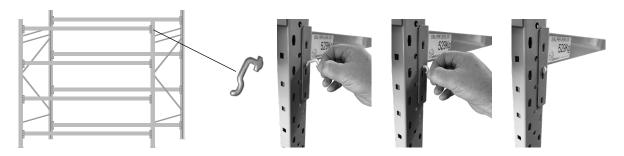
To ensure beams stay securely in place, you must install a beam locking pin into each end of every beam used (every shelf level requires 4 locking pins). Once the beam is located at the correct level and firmly inserted into the tapered post holes, the small hole in the beam indicated below will line up with a matching hole in the post. This will allow the 'S' shaped locking pin to be inserted (thin end first) until the head stops against the beam.
