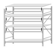
Starting at the bottom level, place the particleboard, wire decks or galvanised shelves onto the top inner lip of each pair of beams as shown in the diagram.
