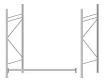
Join the shelf beam to the other frame at the same height. Count the number of slots to make sure they are the same at both ends. Tap into place with a rubber mallet as in step 1.
