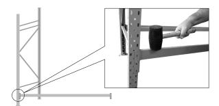
While one person is holding a frame in position, insert the first shelf beam into the frame at the lowest position required. Tap the beam into place near the joint with a rubber mallet. (see diagram).
