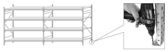
If required, fix frames to the floor through the hole in each foot with appropriate floor fixings (expansion bolts for concrete or screws for wood). Fixings are an optional accessory and not supplied as standard.
