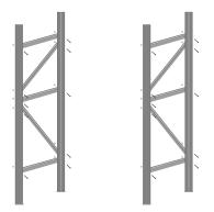
Bolt bracing onto upright posts - (1 upright consists of 2 x posts 2 Diagonal & 3 Horizontal bracing, 10 nuts & bolts).
