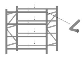
To ensure beams stay securely in place, you must install a beam locking pin into each end of every beam used (every shelf level requires 4 locking pins). Once the beam is located at the correct level and firmly inserted into the tapered post holes, the small hole in the beam indicated below will line up with a matching hole in the post. This will allow the 'L' shaped locking pin to be inserted (thin end first) until the head stops against the beam.
