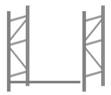
Join the shelf beam to the other frame at the same height. Count the number of slots to make sure they are the same at both ends. Tap into place with a rubber mallet.
