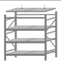
Starting at the bottom level, place the shelving panels onto the top inner lip of each pair of beams as shown in the diagram.
