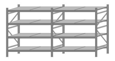
If required, fix frames to the floor through the hole in each foot with appropriate floor fixings (expansion bolts for concrete or screws for wood). Fixings are an optional accessory and not supplied as standard.
