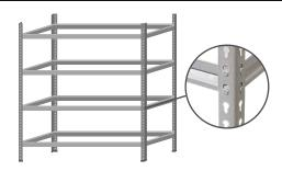
Repeat step 2 to install the other shelf beams. Count the number of slots to make sure the gaps are equal between beams. Once the beam is located at the correct level and firmly inserted into the tapered post holes, the small hole in the beam indicated below will line up with a matching hole in the post.
