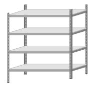
Lay your metal panels on top of each level of support beams. After you have added the remaining shelves and gentle tap on all corners to ensure every beam is in place.
