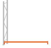
Stand an upright by having one person secure the base or up against wall and lock a beam in at the lowest point.
