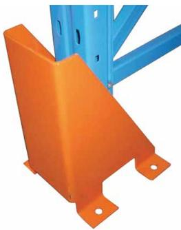
In accordance with the new standards an upright protector (*min 400 mm high*) must be installed at the end of each run to prevent the upright being damaged through an impact.
